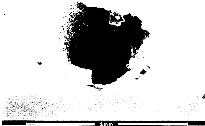
Figure 8. A thru-hole pit on the interior of a tray after ultrasonic cleaning (T134).
