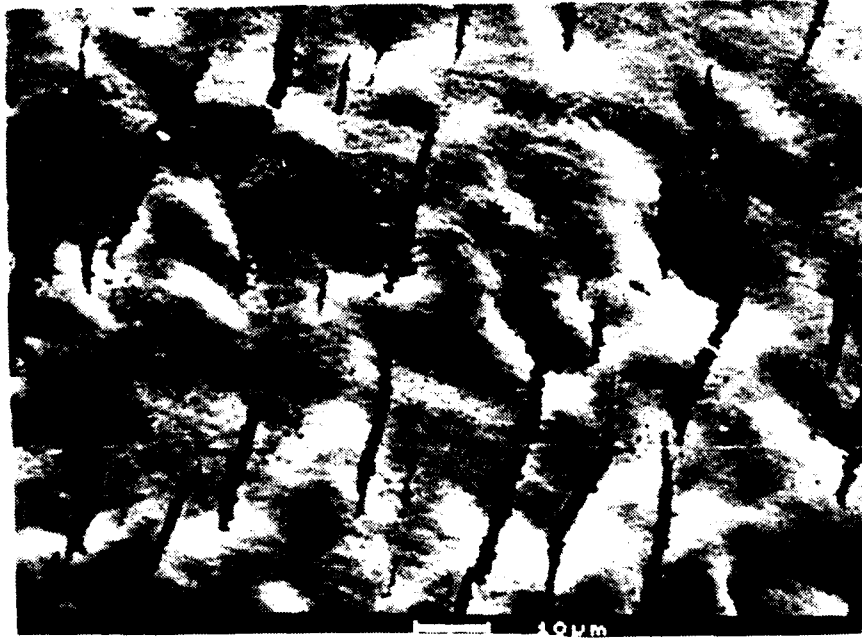
Figure 10. Microcracks in the epoxy layer at the stressed area in the interior of a virgin tray after vinyl topcoat removal.
