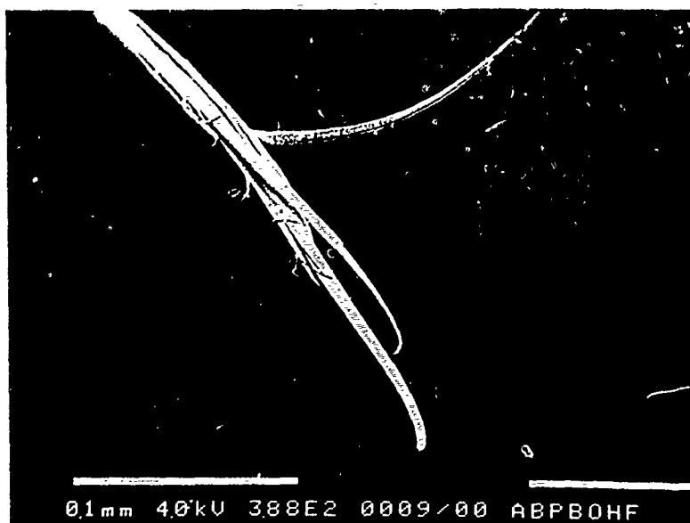
Figure 3.15(b) SEM of HT ABPBO fibre fracture surfaces.
