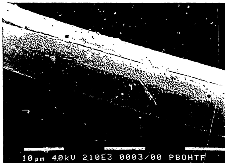
Figure 3.17(b) Cracking along fibre direction in HT PBO fibre.
