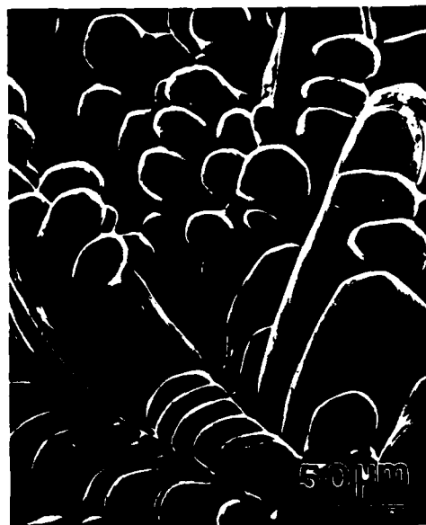
FIG. 2. Hexagonal dendrite in the shrinkage cavity of a Ti-50at%Al alloy arc-melted button. Note the striations along the basal plane arising from the solid state transformation of \alpha into the \alpha_2 + \gamma lath microconstituent.
