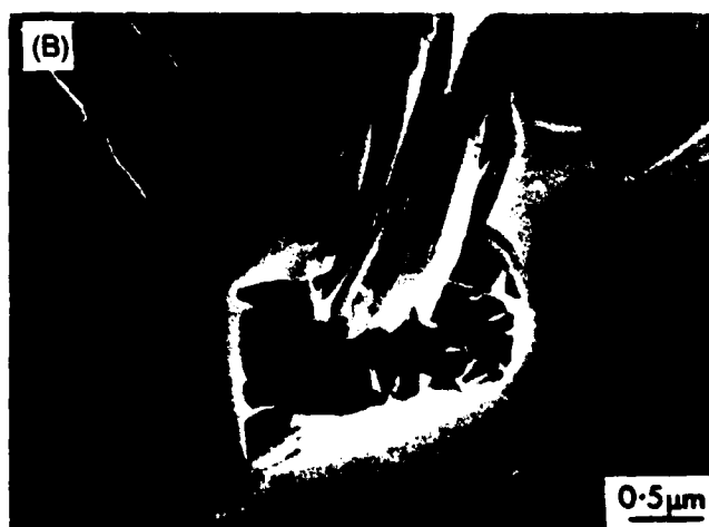
Fig. 8. (A) Scanning electron micrograph and schematic illustration of a sintered SiC fracture face of a bend beam deformed at a temperature above the transition and then fractured at room temperature. (B) Creep damage void nucleated at a graphite inclusion near the blunt indentation crack.
