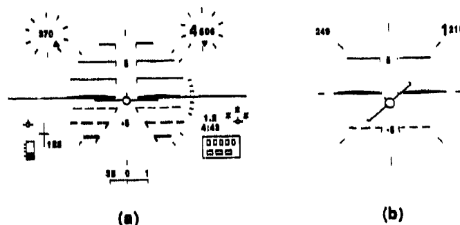
Figure 3. Prototype HUD displays which follow the guidelines listed in text. A full-format display is shown in (a), while a decluttered one is shown in (b). (Reproduced from [4].)
