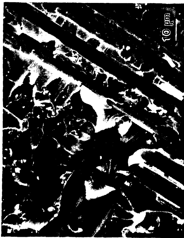
Figure 4.11 Interlaminar cracking at the edge of a \pm 45^\circ angle-ply specimen. (a) Overview (b) Close-up of the same area
