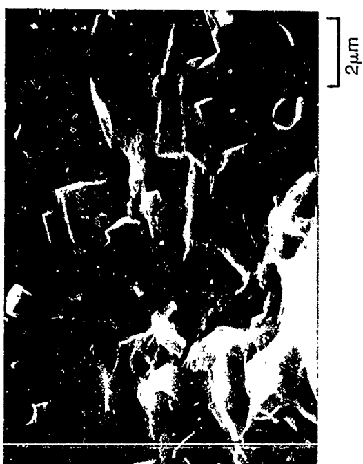
Fig. 14 Fracture Surface of LAS-I Matrix/BN Coated Arco SiC Whisker Composite #335-89
