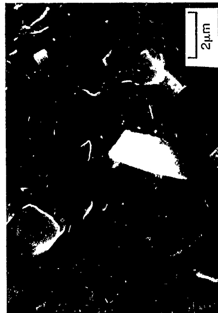
Fig. 8 Fracture Surface of LAS-I Matrix/Tokai TWS-400C Carbon Coated SiC Whisker Composite #309-89
