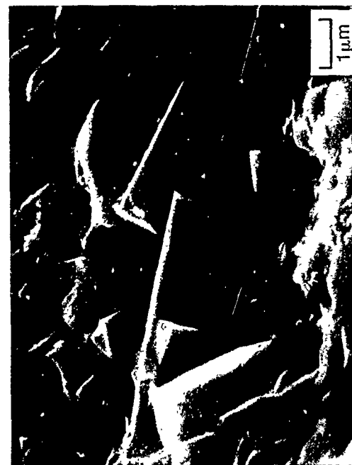
Fig. 19 Fracture Surface of CAS Matrix/Tokai TWS-400 SiC Whisker Composite #499-89
