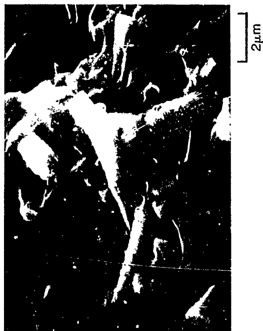
Fig. 14 Fracture Surface of LAS-I Matrix/BN Coated Arco SiC Whisker Composite #335-89
