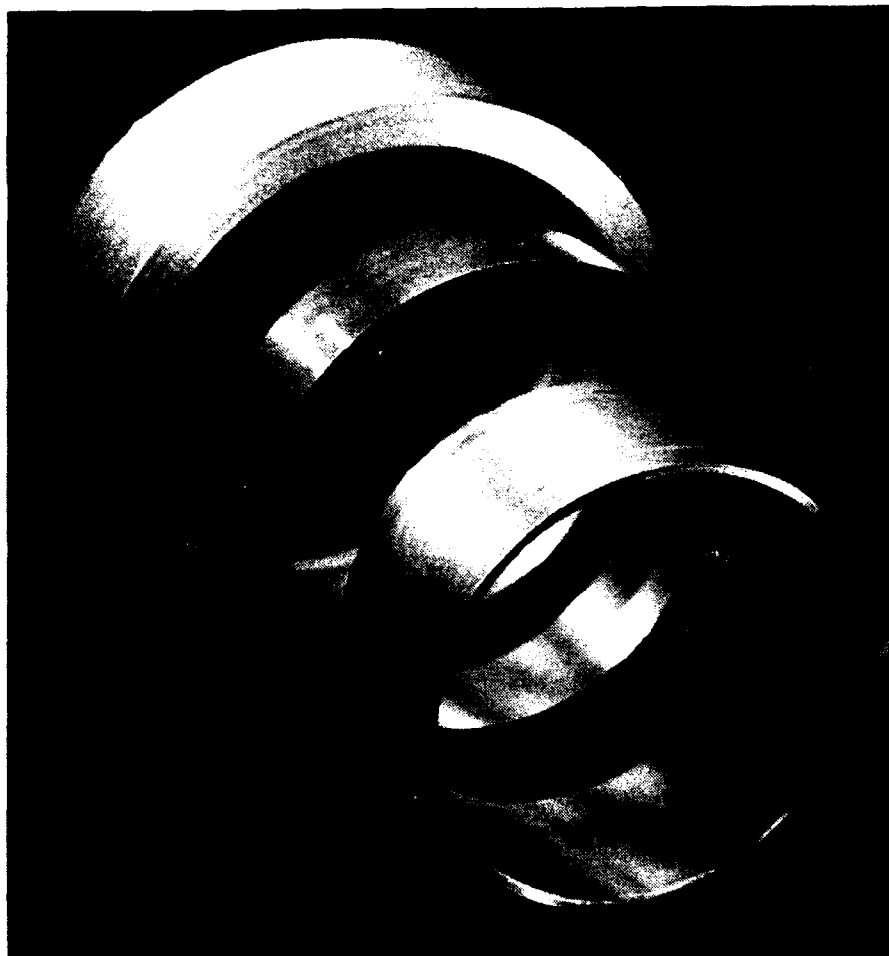
Figure 4.5.4.2.5 Elements of MMC hoop nesting trial prior to assembly and HIP.
