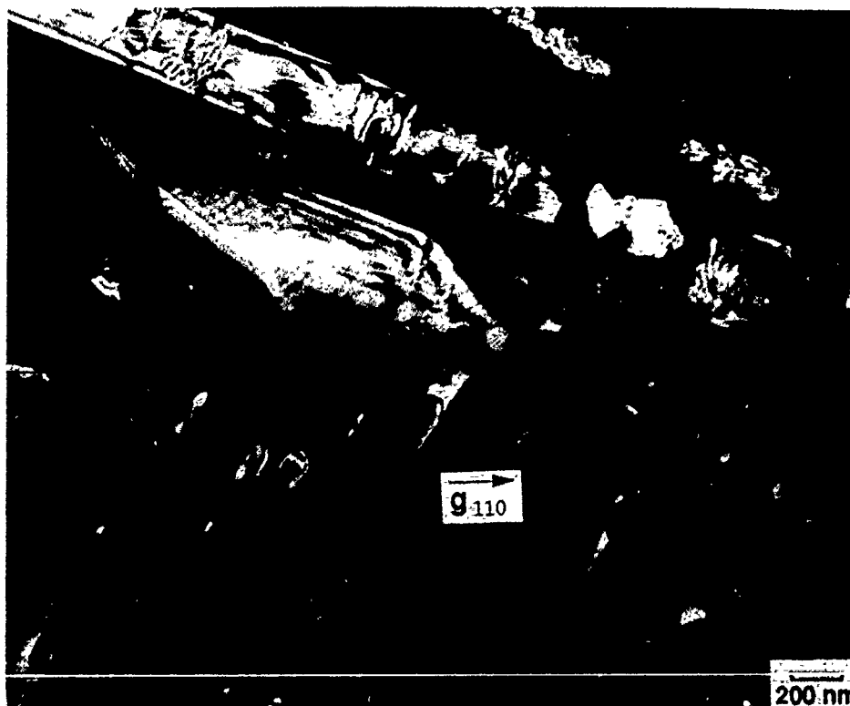
Figure 3-75 (a) Bright-field TEM micrograph of specimen in Figure 3-73 showing a region with coarsened precipitates within the \alpha -2 phase which light up in the dark-field micrograph (b) imaged with the (110) \beta diffraction vector.
