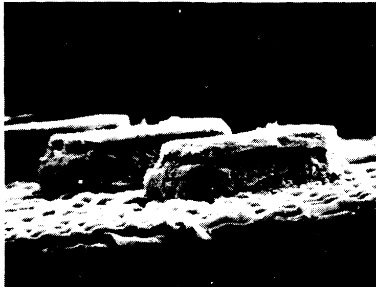
Figure 2-16. Failure Analysis of Interconnect Loss on a 240x80 Format FPA Shows Failure at the Indium Column/HgCdTe Interface
