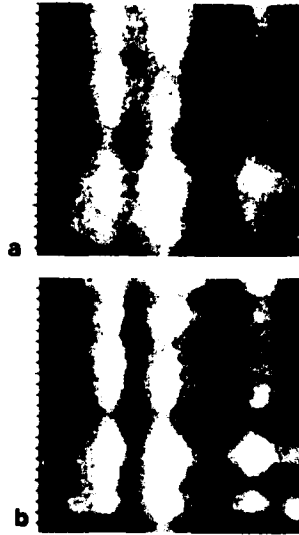
Figure 4 a Internal images of the cure cracks in a graphite/epoxy composite. Figure 4 b Result of Wiener filtering the image in Figure 4 a using a PSF obtained by C-scanning a ball bearing.
