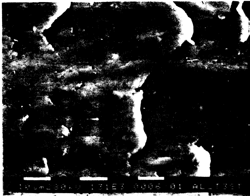
Figure 9. SEM micrograph of scratch surface after 10,000 cycles, 1300 magnification
