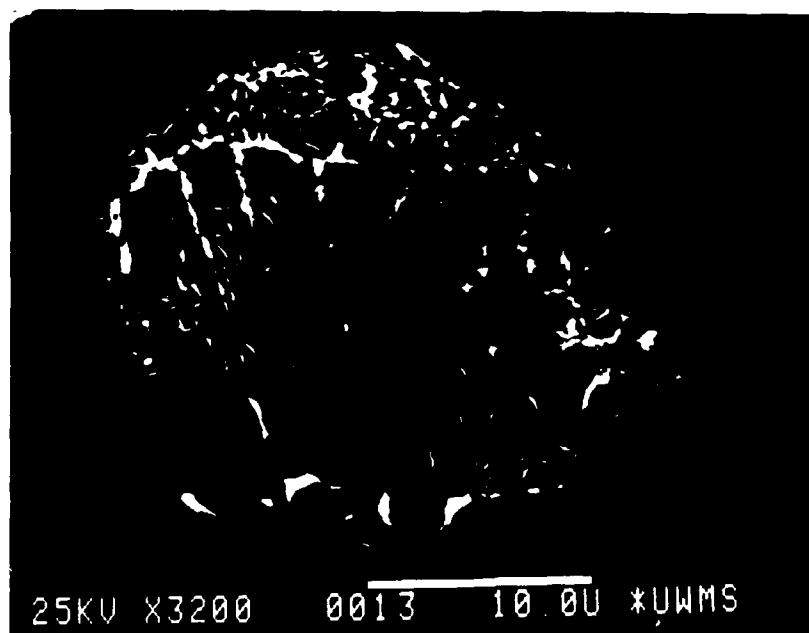
Figure 45. SEM micrographs of Nb-33 at. % Al showing microstructural development in 20-37 \mu\text{m} powder following drop tube processing.
