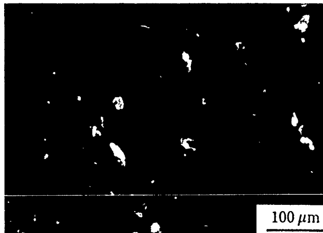
Fig 14 SIMS map using sodium ions of fracture surface of 25mm plate showing (bright) sodium-rich areas. Surface diffusion of sodium has probably occurred after fracture prior to analysis so that the areas are much larger than the original phases
