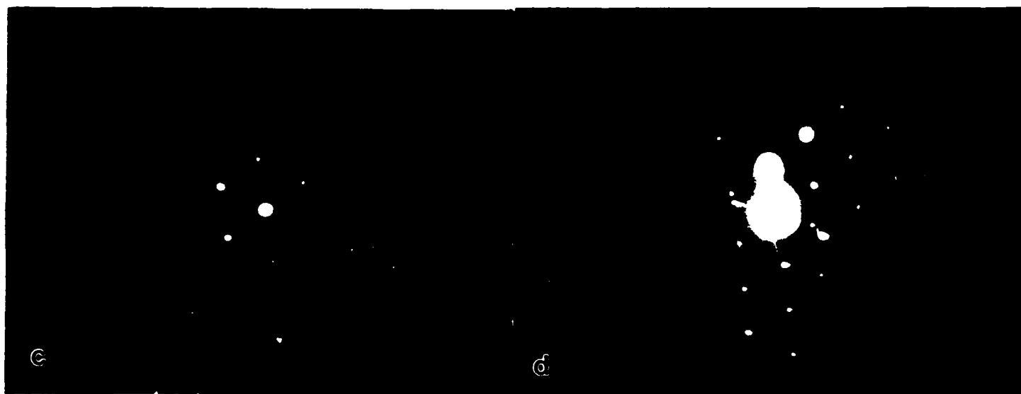
(b) Dark field micrograph taken from (002) spot. Needle like features can be seen at the interface. (c) Near zone axis (110) diffraction pattern. (d) Diffraction pattern showing spots from the reaction products on tilting slightly off from the (110) zone-axis.
