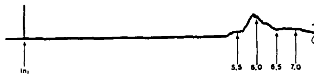
FIGURE 4: HPLC Chromatogram of Base Extracted JP-5 Jet Fuel from Iorizaki, Japan.
