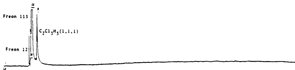
Fig. 3: GC of CS 2 Extract From Rear Section of Carbon Sorbent Tube (Sample A7-7-1R)
