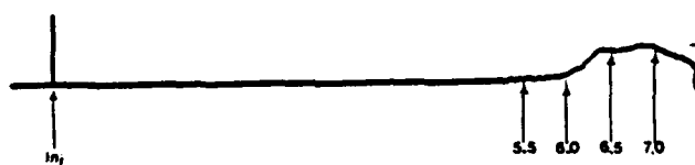
FIGURE 6: HPLC Chromatogram of Base Extracted JP-5 Jet Fuel From Cartagena, Spain.
