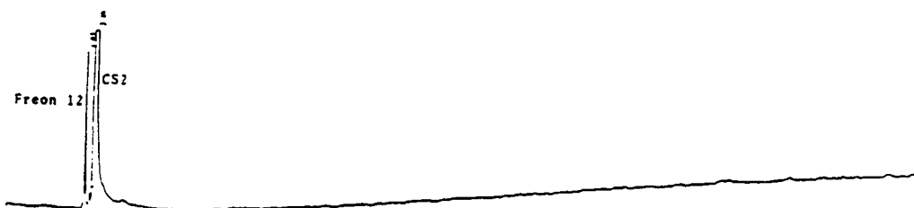
Fig. 2: GC of CS 2 Extract From Front Section of Carbon Sorbent Tube (Sample A7-7-1F)
