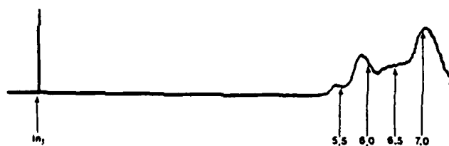
FIGURE 2: HPLC Chromatogram of Base Extracted JP-5 Jet Fuel from Guantanamo, Cuba.
