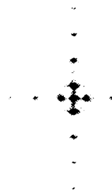
Figure 4.7. Simple texture image of two orientations at 10 cycles/cm, and its Fourier transform
