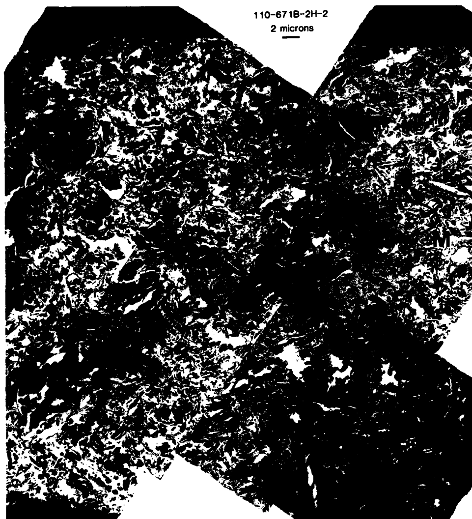
Figure 22.5(a-c). TEM photograph mosaics of Sample 671B-2H-2 (8.9 mbsf). Porosity: 76%. This unoriented sample exhibits an open structure of randomly oriented domains (M, matrix) surrounding biogenic particles (B), such as foraminiferal tests and nannofossils, and fractillites (F). Possible dewatering paths are indicated by channels (C) and by pore spaces with face-to-face arranged particles forming a rim around the pathway (W).
