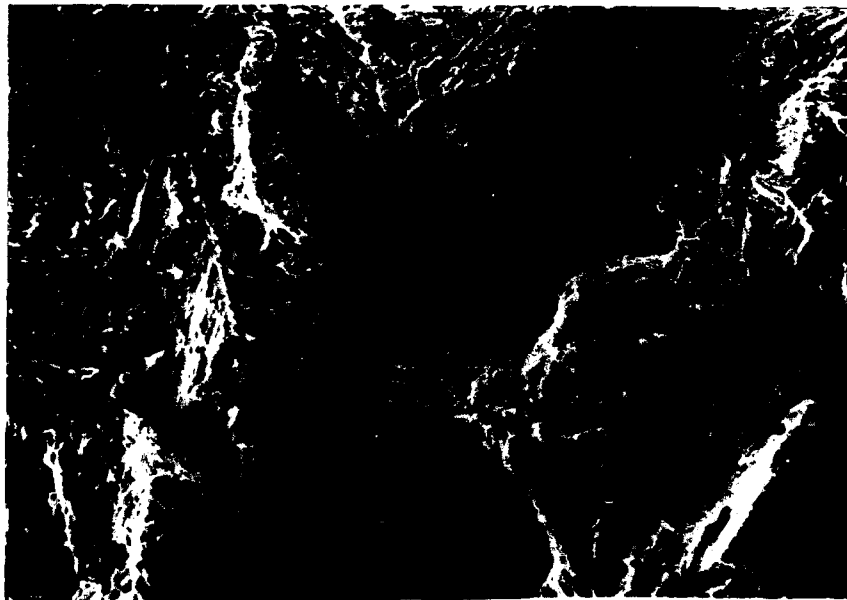
Fig.4.47. Quasi-cleavage fracture mode with river patterns and tear ridges indicating the influence of martensite in DQ-125; 500X
