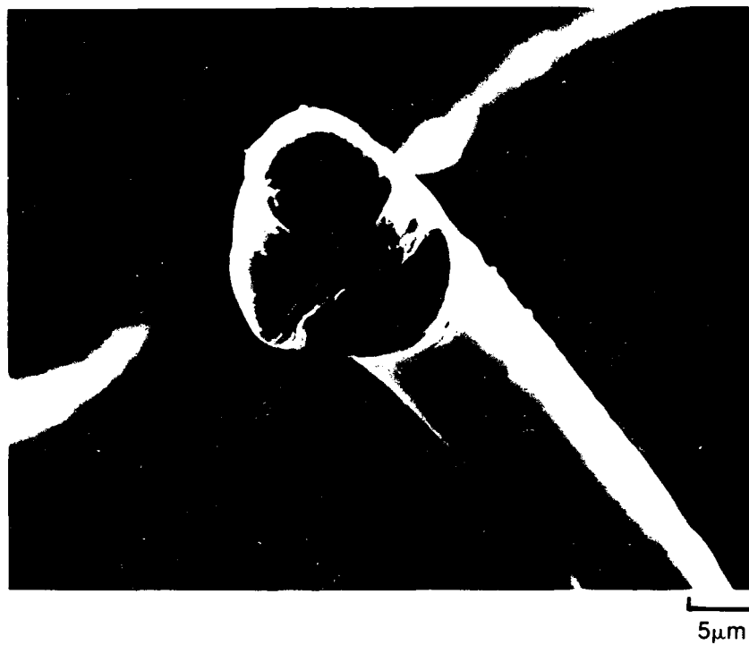
FRACTURED END OF A LOT 9217-53C1 DOW CORNING SiC FIBER UTS=58 ksi (400 MPa)
