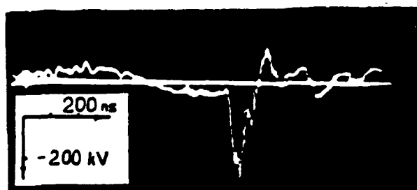
c: Shape of the high voltage pulse.
