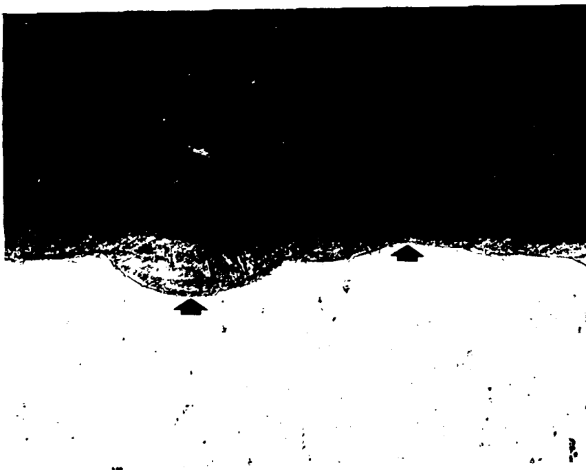
Figure 25. Metallographic cross section of a Hastelloy X laser machined surface showing recast layer variability. The recast layer of adjacent areas varies form .0005" to .0044" (arrows). Mt. No. 90-477, Mag: 100X, Etchant: Glyceregia
