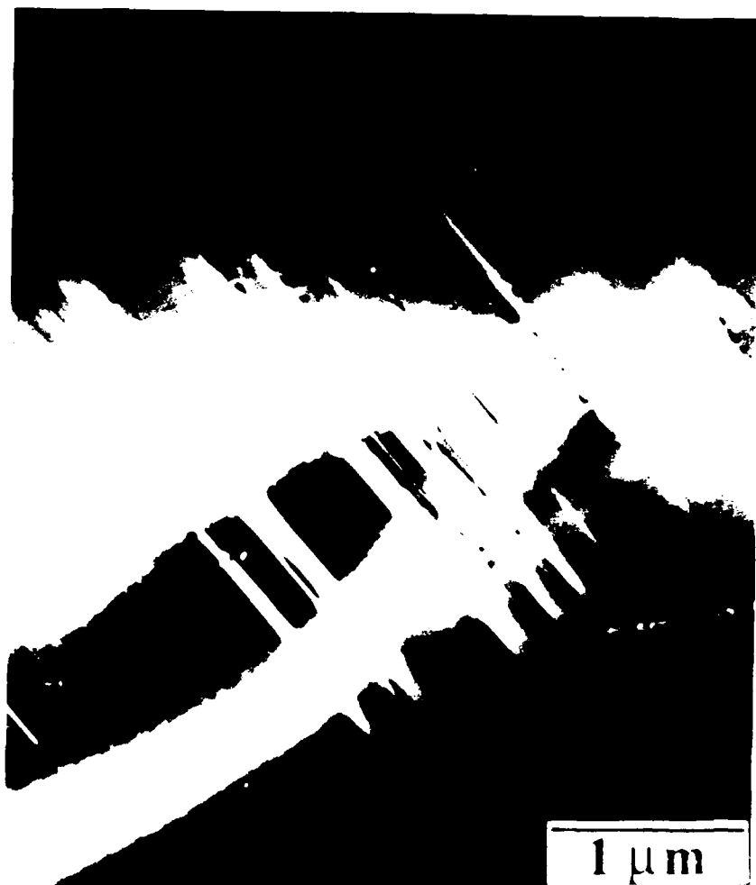
Figure 2 Transmission electron micrograph of as-arc-cast \text{Al}_{0.75}\text{Ti}_{0.25}\text{Fe}_{0.5} alloy, showing a large faulted precipitate.
