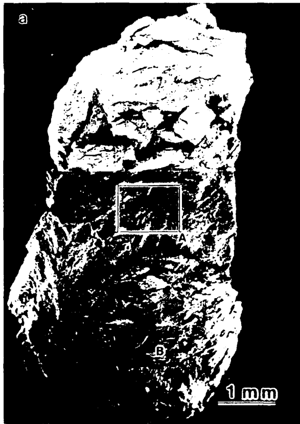
Figure 12 Deformed specimens in compression at room temperature. (a) annealed for homogenization; (b) HIPed.
