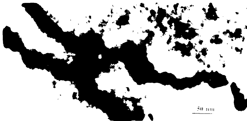
Figure 3 Dark field micrograph of a homogenized \text{Al}_{67.5}\text{Ti}_{25}\text{Fe}_{7.5} specimen, showing tiny precipitates on dislocations. A 111 L1_2 reflection has been used.
