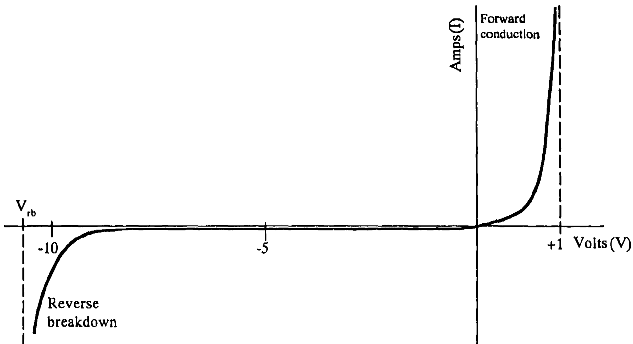
Fig. 2 - Metal semiconductor junction I-V characteristic showing reverse breakdown
