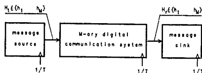
Fig. 2.1.1. Basic structure of the M-ary communication system
