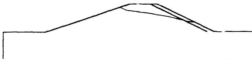
e) levee with 1-ft layer of permeability , k_1 and k_1 / k_2 = 0.1
