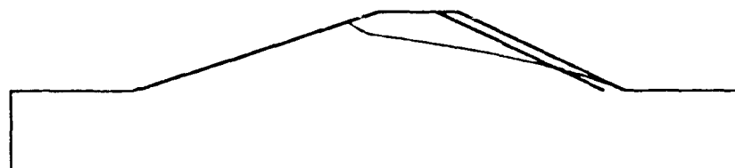
d) levee with 1-ft layer of permeability , k_1 and k_1 / k_2 = 10
