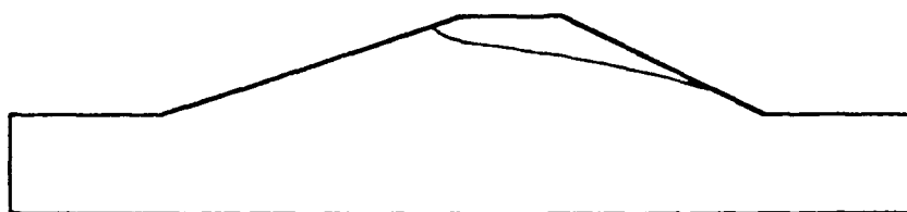
a) levee with constant permeability , k_2
