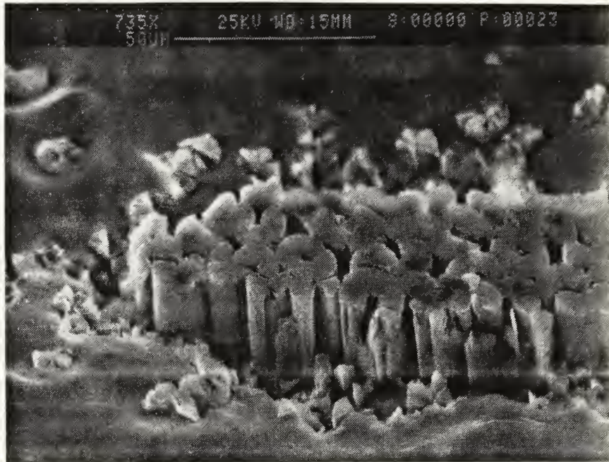
Figure 13: SEM micrograph of an unprotected edge sample immersed in 3.5% sodium chloride for 14 days. The sample is tilted 45 degrees. (735X)
