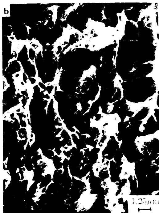
Fig. 5. Fracture surface morphology of the unreinforced control alloy: a—showing the distribution of the large dimples and b—showing the distribution of the small dimples.
