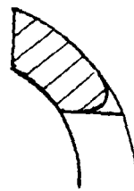
FIGURE 11: DETAILS OF AUXILIARY INTAKE LIP GEOMETRY.
