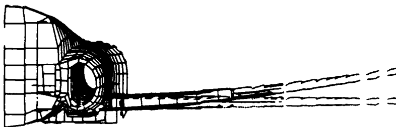
Figure 2.5. T-38 Structural Deformations
