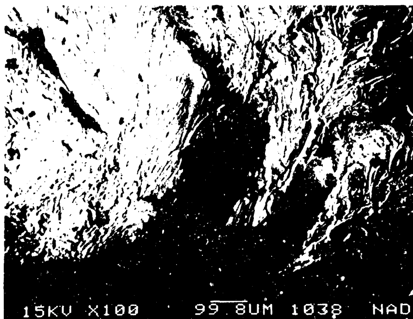
b. Backscatter SEM Micrograph of Foreign Material
