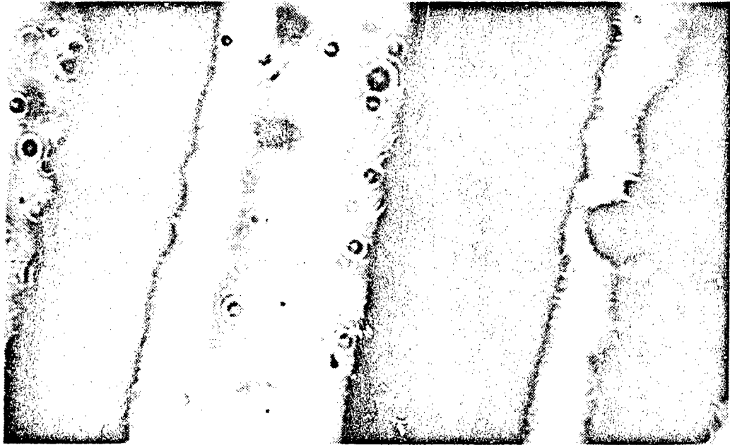
A-18 Autoradiogram, Teflon-coated Nomex seam exposed to carbon-14 labeled methylene chloride for 75 minutes. The double Teflon layer (2 dark lines) about 380 \mu\text{m} from the chemically exposed side are seen. Some autoradiographic silver grains (black specks) are visible. Transmitted bright field (1600x).
