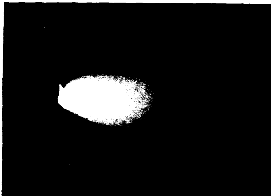
Figure 4.5. Plasma formation in a UHV chamber. (Energy = 2.3 \times 10^{-1} joule)
