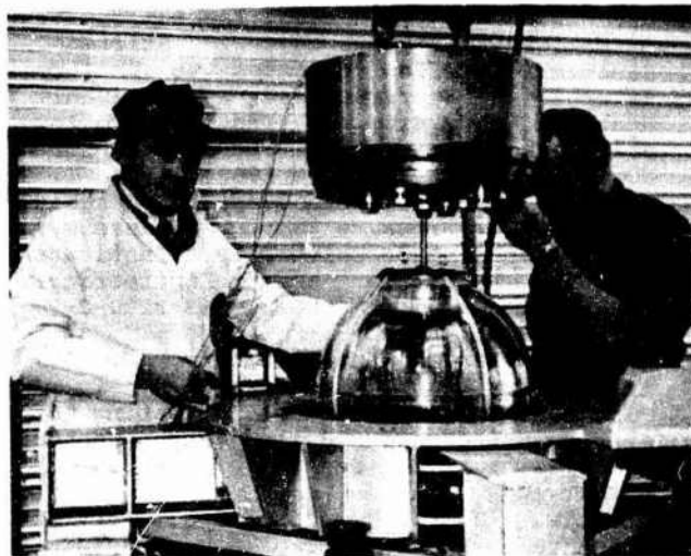
Figure 27 Typical arrangement for hydrostatic testing of acrylic plastic spherical hull scale models. The spherical hulls are suspended from the pressure vessel end closure by means of a pipe open at one end to the interior of the hull and on the other end to the exterior of the vessel. This tube served as pressure resistant conduit for instrumentation wires and relief for internal pressure buildup in the sphere.
