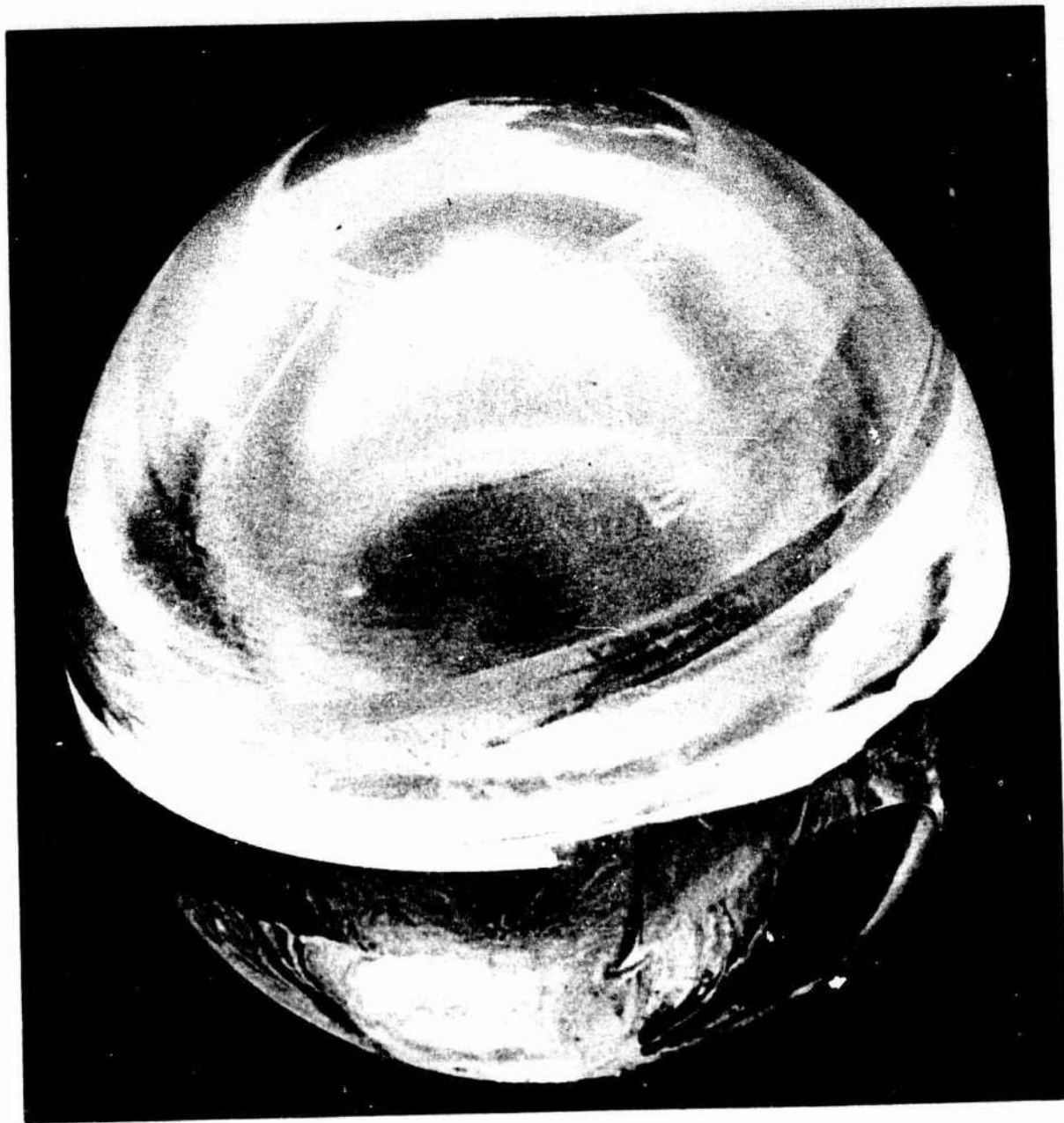
Figure 17. Fracturing in cast acrylic sphere after 20,000-psi external hydrostatic pressure for 1 hr. The cracks formed during depressurization. View of bottom hemisphere.
