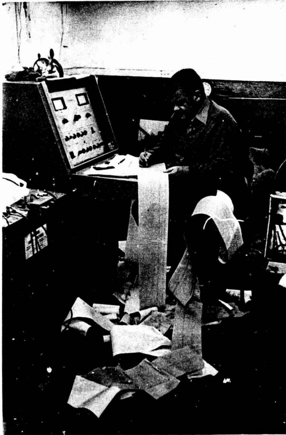
Figure 14. Dynamic strains and ram displacement were recorded on paper moving at 32 inches/second.
