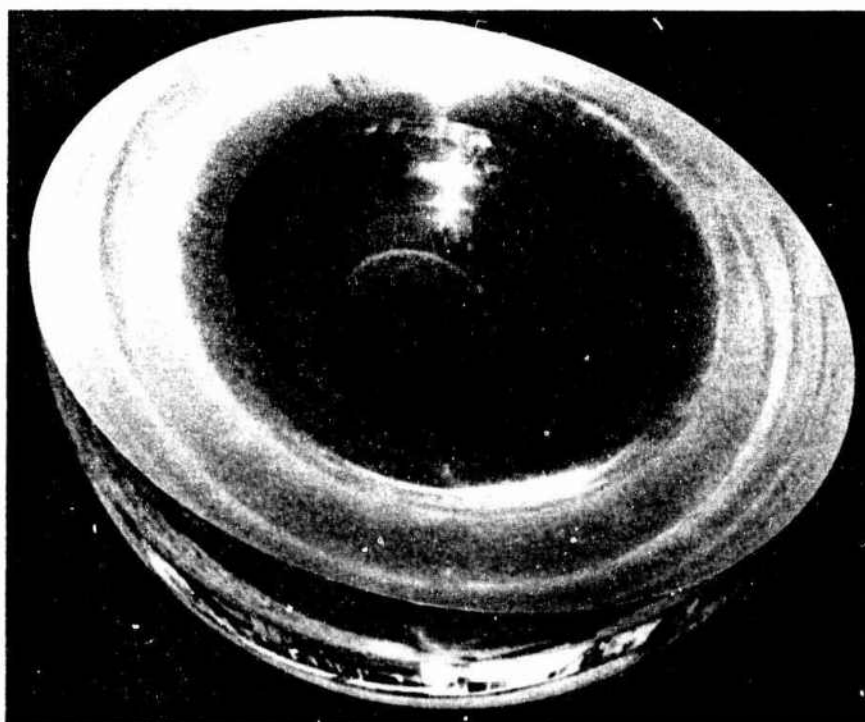
Figure 21. Spherical specimen 3 after 100 pressure cycles to 5000-psi hydrostatic pressure. Note complete absence of cracks.
