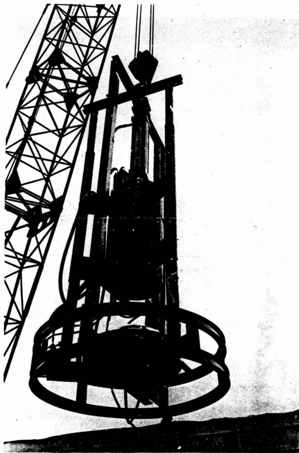
Figure 9. Impact loading ram assembly prior to placement in the SWRI pressure vessel.
