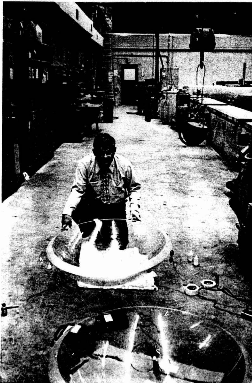
Figure 5. Typical acrylic plastic spherical sector window with R_0 = 24 inches, t = 2.25 inches and \alpha = 117^\circ used as a test specimen in the impact loading study.
