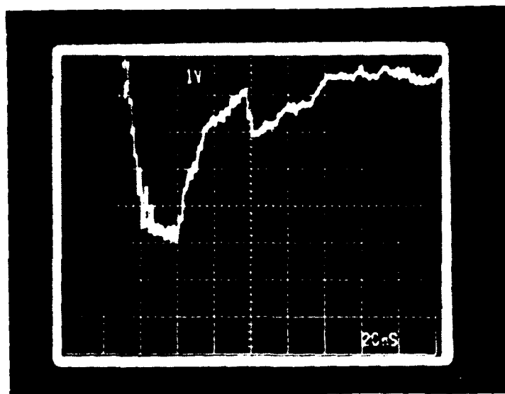
Figure A.13 Typical diode voltage waveform for a 75 kV shot (46 dB attenuation at oscilloscope).
