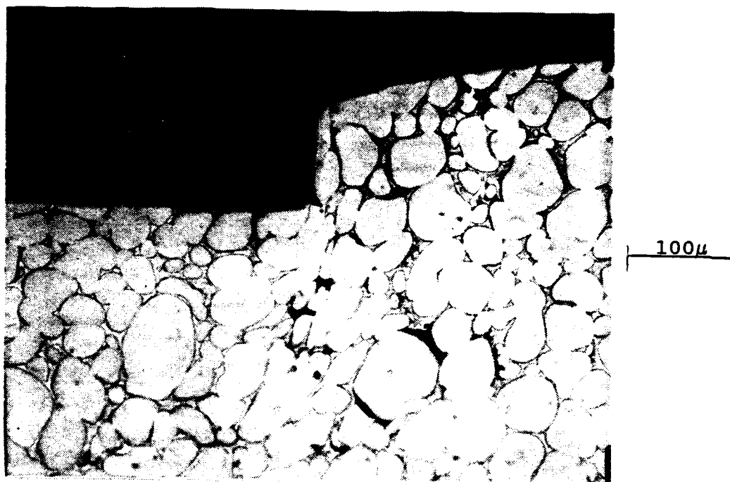
Figure 25. Region of the Punch Strike, #71, LPS 90%W, 500°F
