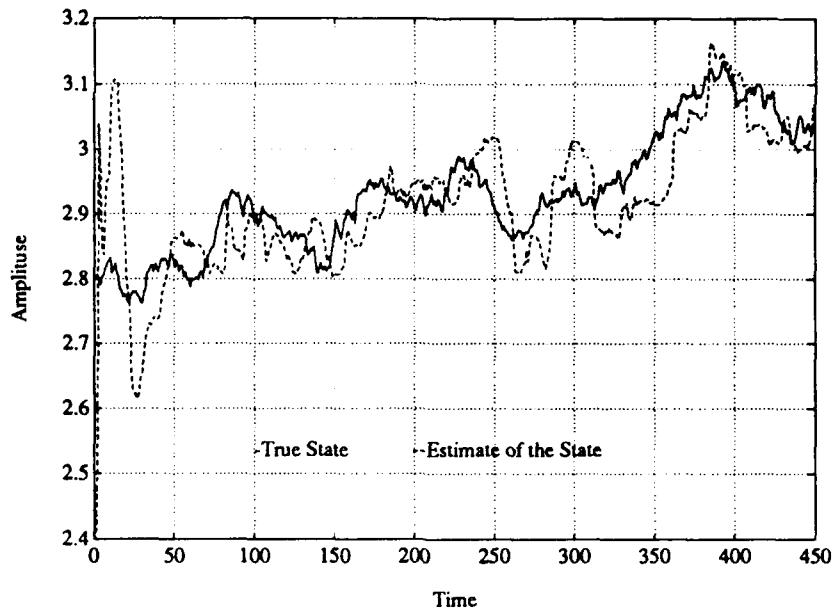
Figure 5.10 Amplitude tracking of the first harmonic. (Three harmonic case)
