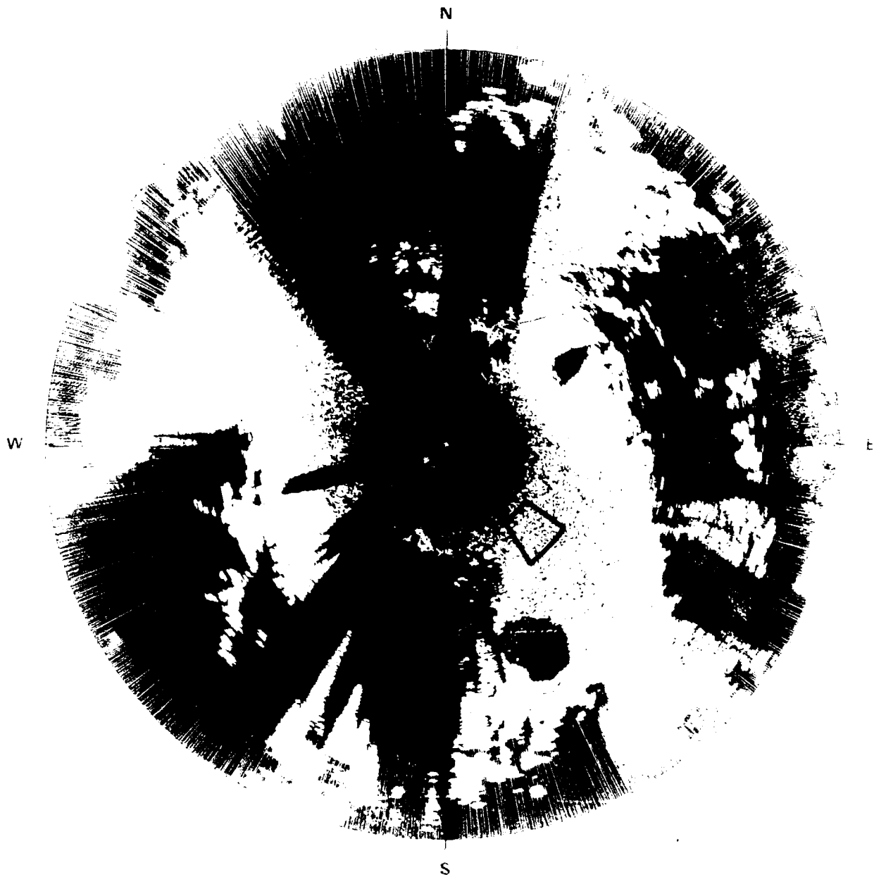
Figure E-154. PPI clutter map and repeat sector at Booker Mountain. Repeat sector is outlined in black. Maximum range = 48.4 km. X-band, 150-m pulse, horizontal polarization; cells with \sigma^0 F^4 \geq -40 dB are white.
