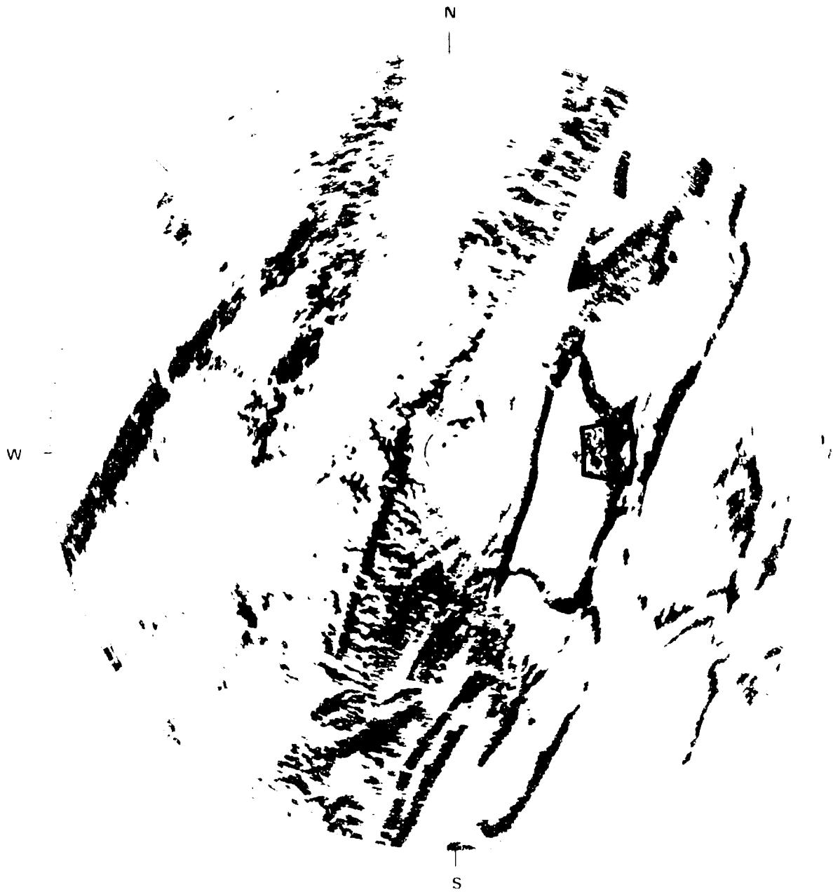
Figure E-37. PPI clutter map and repeat sector at Blue Knob. Repeat sector is outlined in black. Maximum range = 48.4 km; X-band, 150-m pulse, horizontal polarization; cells with \sigma^0 F^1 \geq -40 dB are red
