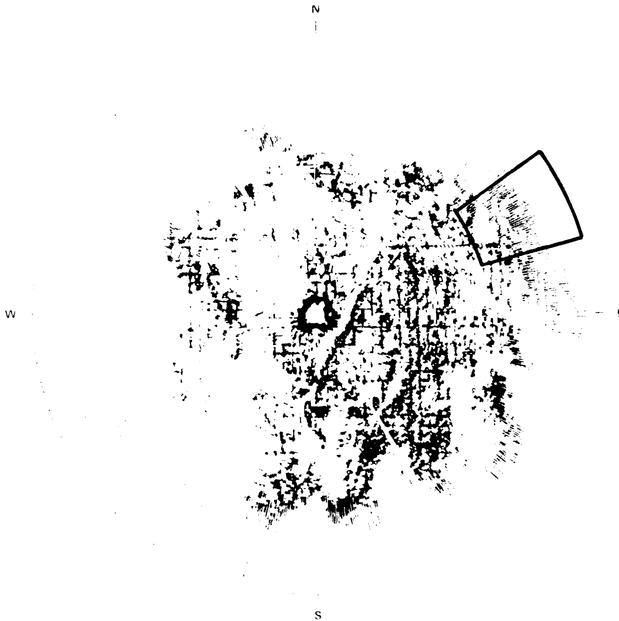
Figure E-55. PPI clutter map and repeat sector at Penhold II. Repeat sector is outlined in black. Maximum range = 25 km; S-band, 150-m pulse, horizontal polarization; nominally, cells with \sigma^0 F^4 \geq -50 dB are red, but precise threshold is unknown due to uncertain calibration.
