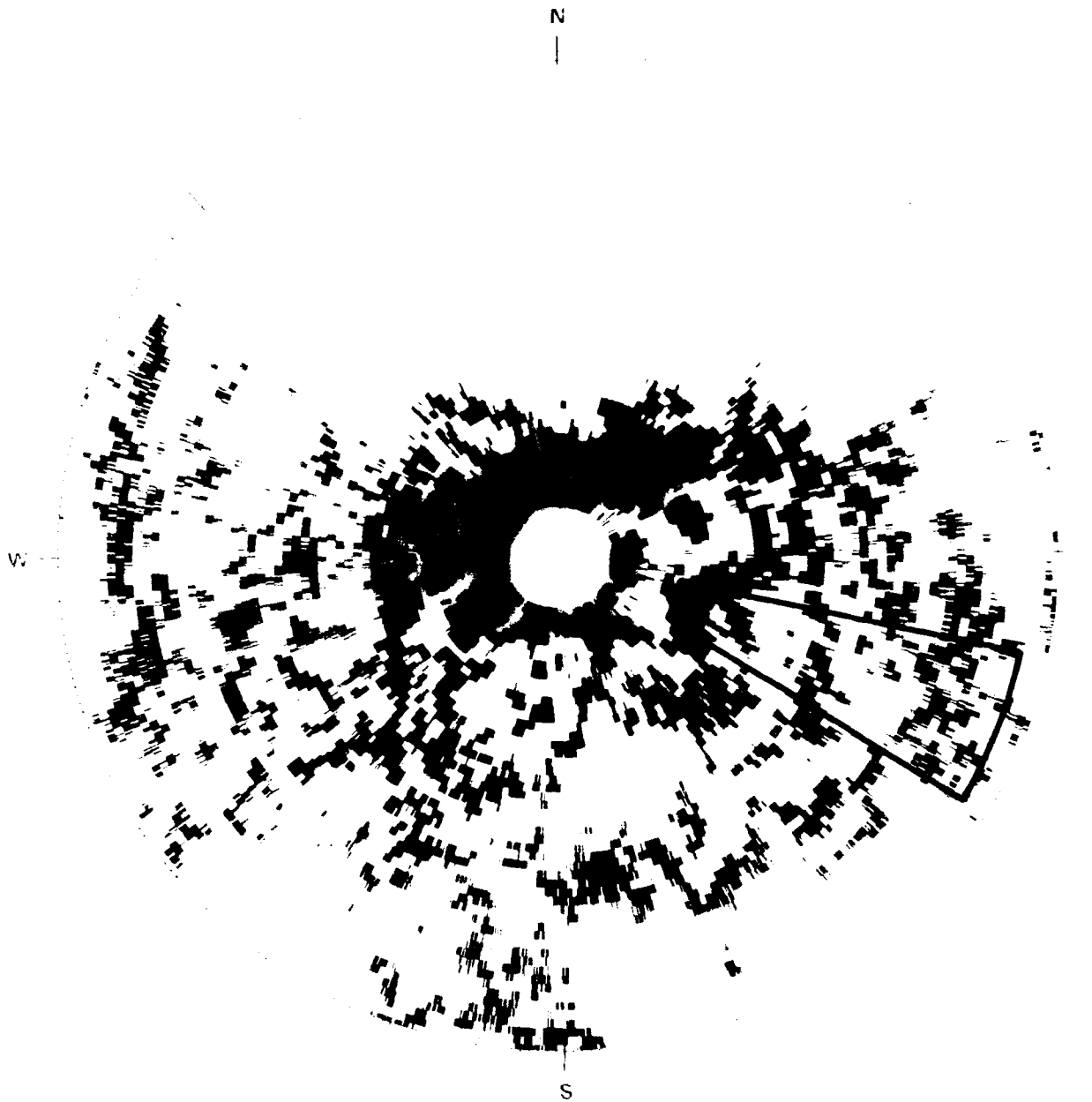
Figure E-80. PPI clutter map and repeat sector at Turtle Mountain. Repeat sector is outline in black. Maximum range = 8.5 km; X-band, 150-m pulse, horizontal polarization; cells with \sigma^0 F^4 \geq -40 dB are red
