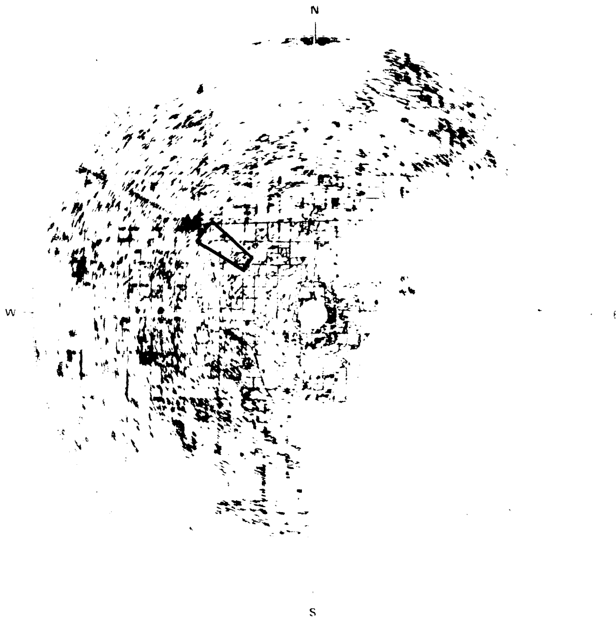
Figure E-132. PPI clutter map and repeat sector at Wolseley. Repeat sector is outlined in black. Maximum range = 20 km; X-band, 15-m pulse, horizontal polarization; cells with \sigma^{\circ}F^4 \geq -45 dB are red.
