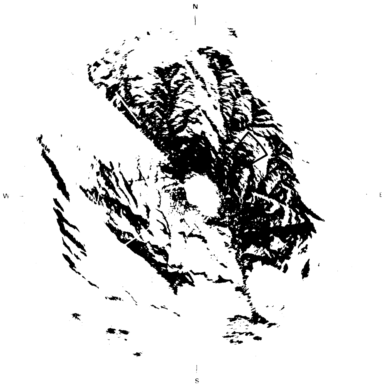
Figure E-158. PPI clutter map and repeat sector at Vananda East. Repeat sector is outlined in black. Maximum range = 20 km; X-band, 15-m pulse, horizontal polarization; cells with \sigma^0 F^4 \geq -40 dB are red.
