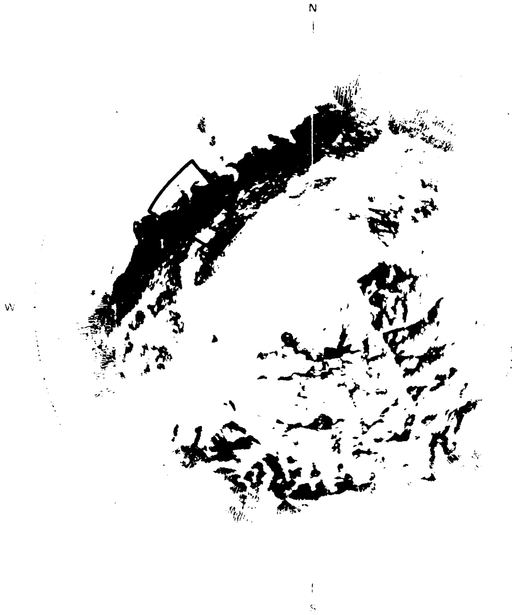
Figure E-41 PPI clutter map and repeat sector at Scranton. Repeat sector is outlined in black. Maximum range = 20 km, S band, 15-m pulse, horizontal polarization, cells with \sigma_{FH} \geq -40 dB are red
