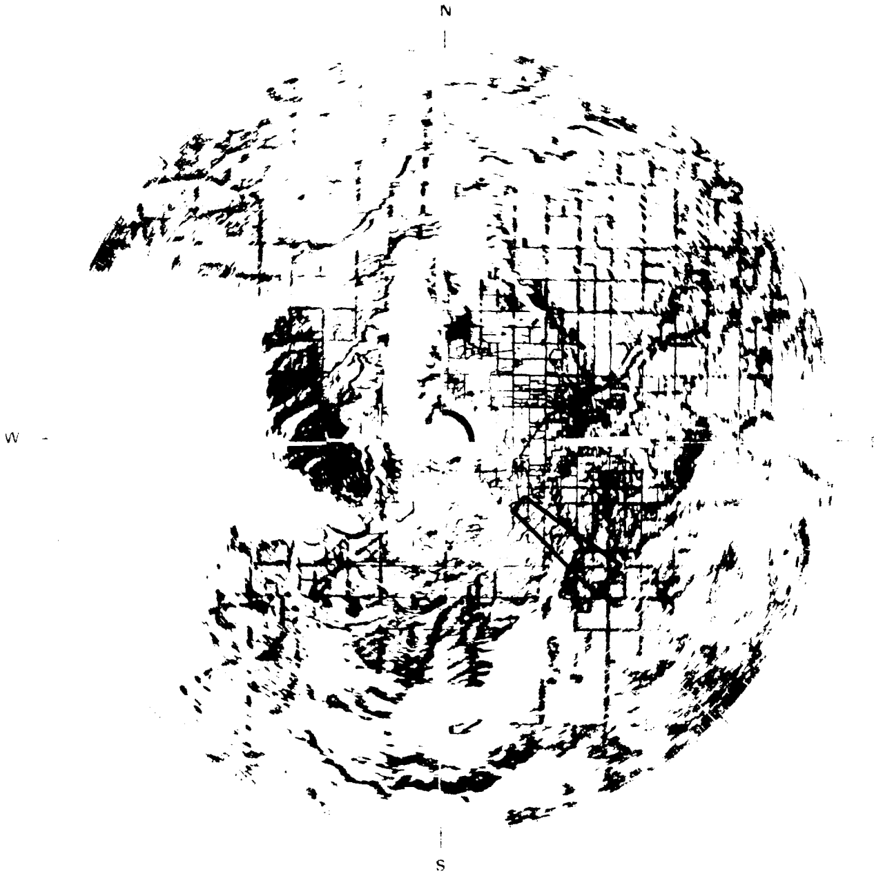
Figure E-114. PPI clutter map and repeat sector at Magrath. Repeat sector is outlined in black. Maximum range = 20 km; X-band, 15-m pulse, horizontal polarization; cells with \sigma^0 F^4 \geq -40 dB are red.
