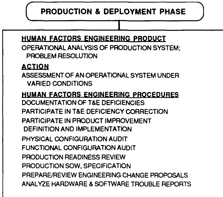
Figure 7. Human Factors Engineering Product, Action, and Procedures Related to the Production and Deployment Phase of the Weapon System Acquisition Cycle, Following Milestone 3.
