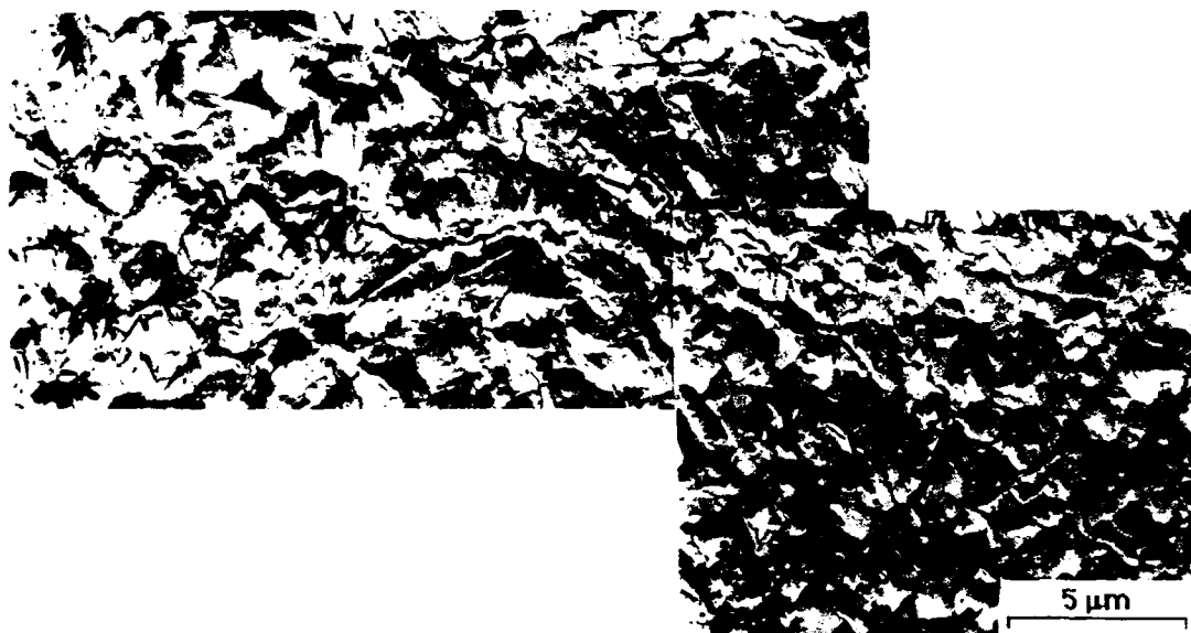
Fig. 14. TEM replica showing inhomogeneously distributed microcracks and grain-boundary cavities associated with creep-crack growth in pyroceram.
