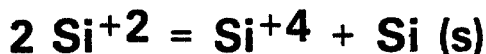
Figure 5. Proposed mechanism for formation of fine Si precipitates in Mg-Si-Al-O-N glasses from Geld and Esin. 17
