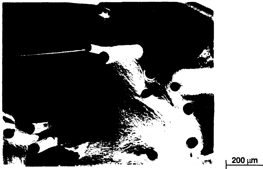
Figure 4-19. SEM photomicrograph showing evidence of localized softening or melting of the glass-ceramic matrix. From a specimen subjected to a thermomechanical fatigue profile including a 60 sec. hold at \sigma_{\max} . Mag: 400X
