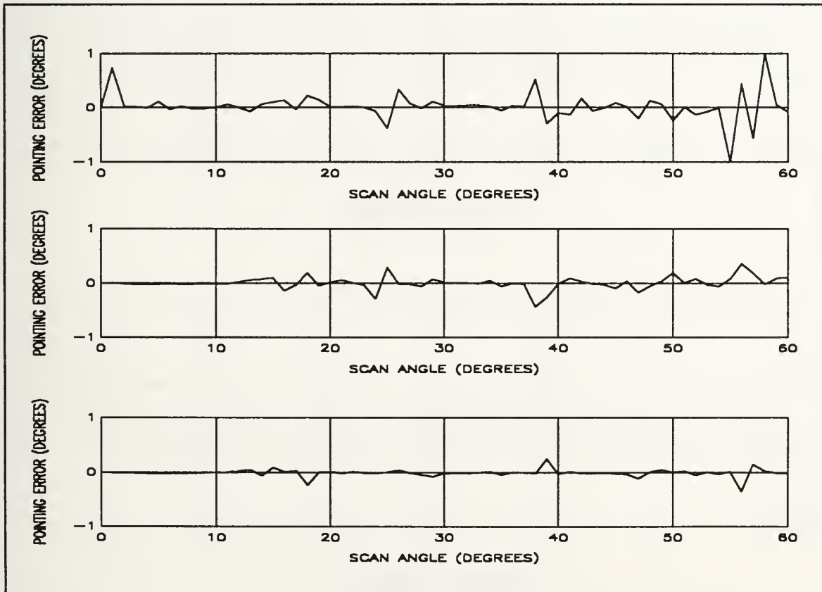
Figure 63. Pointing Error versus Scan Angle for 26 Element Arrays with 3, 4, and 5 Bit Phase Shifters using Regular Roundoff
