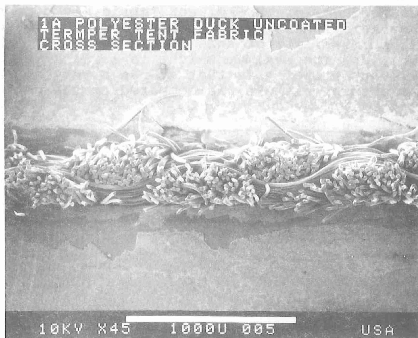
Figure 5: SEM photograph of a yarn of polyester duck showing gaps between fibers. (Mag. x45)
