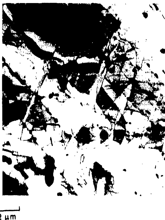
Figure 49. Electron Micrograph of Alloy 993 (SCWA-211) Tensile Tested at 705°C (1300°F). Note Rod-Like Precipitates
