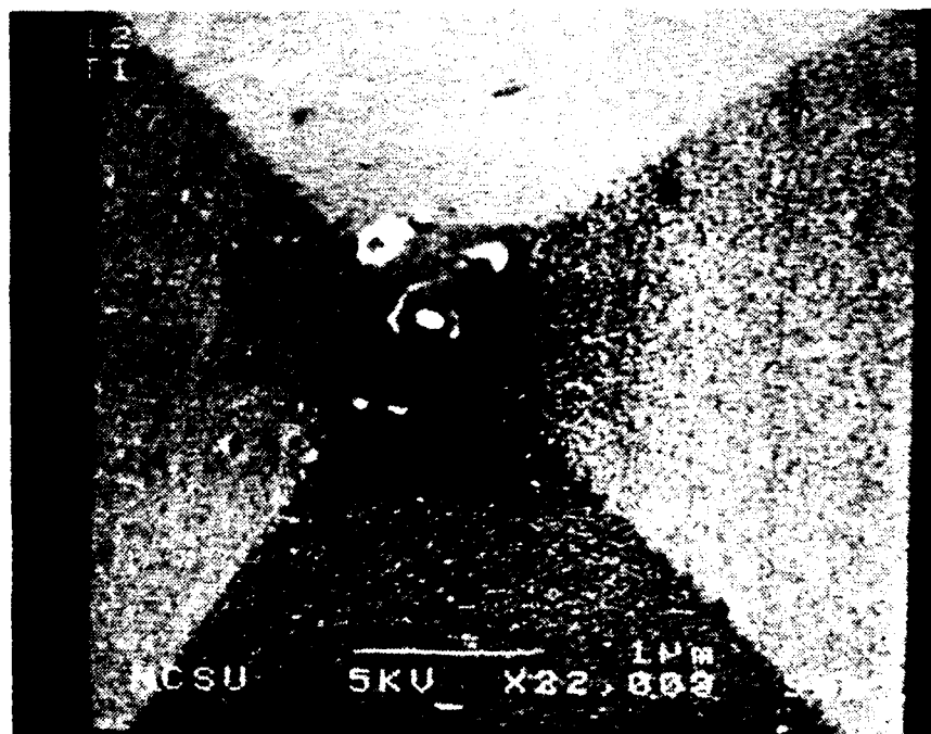
Figure 23: Microtip that was grown with improper stigmation. Note that it is elliptical instead of circular.
