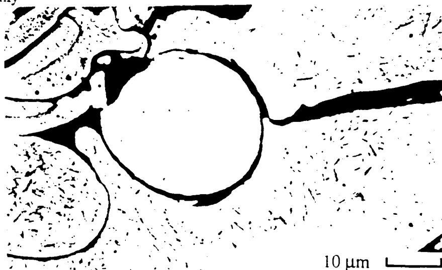
Fig. 11. SEM microphotograph of the sprayed 0.8% C steel: Showing martensite formation surrounded by retained austenite. The martensite particles are acicular in appearance in this section (probably being lenticular in three dimensions) and vary in size: they are of the order of 0.5 \mu\text{m} by 4 \mu\text{m} .
