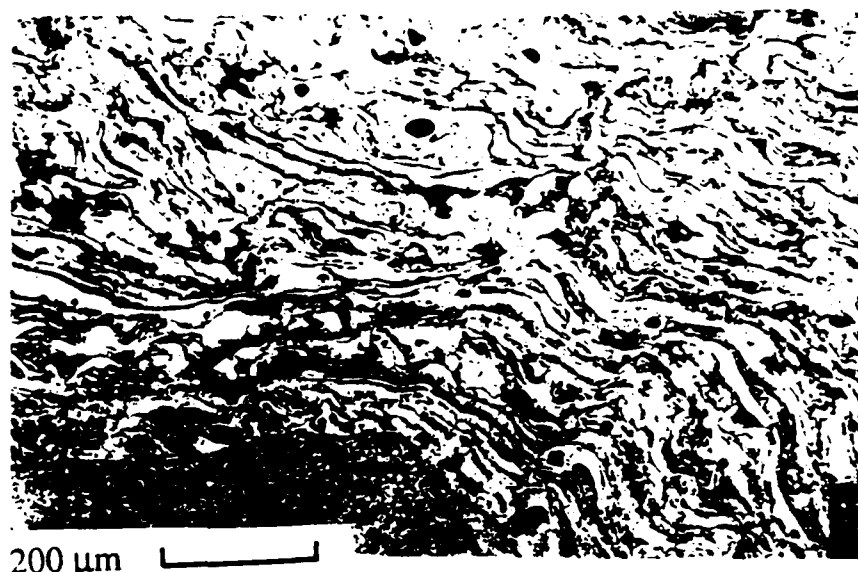
Fig. 20. Flow of oriented lamellæ around corner.
