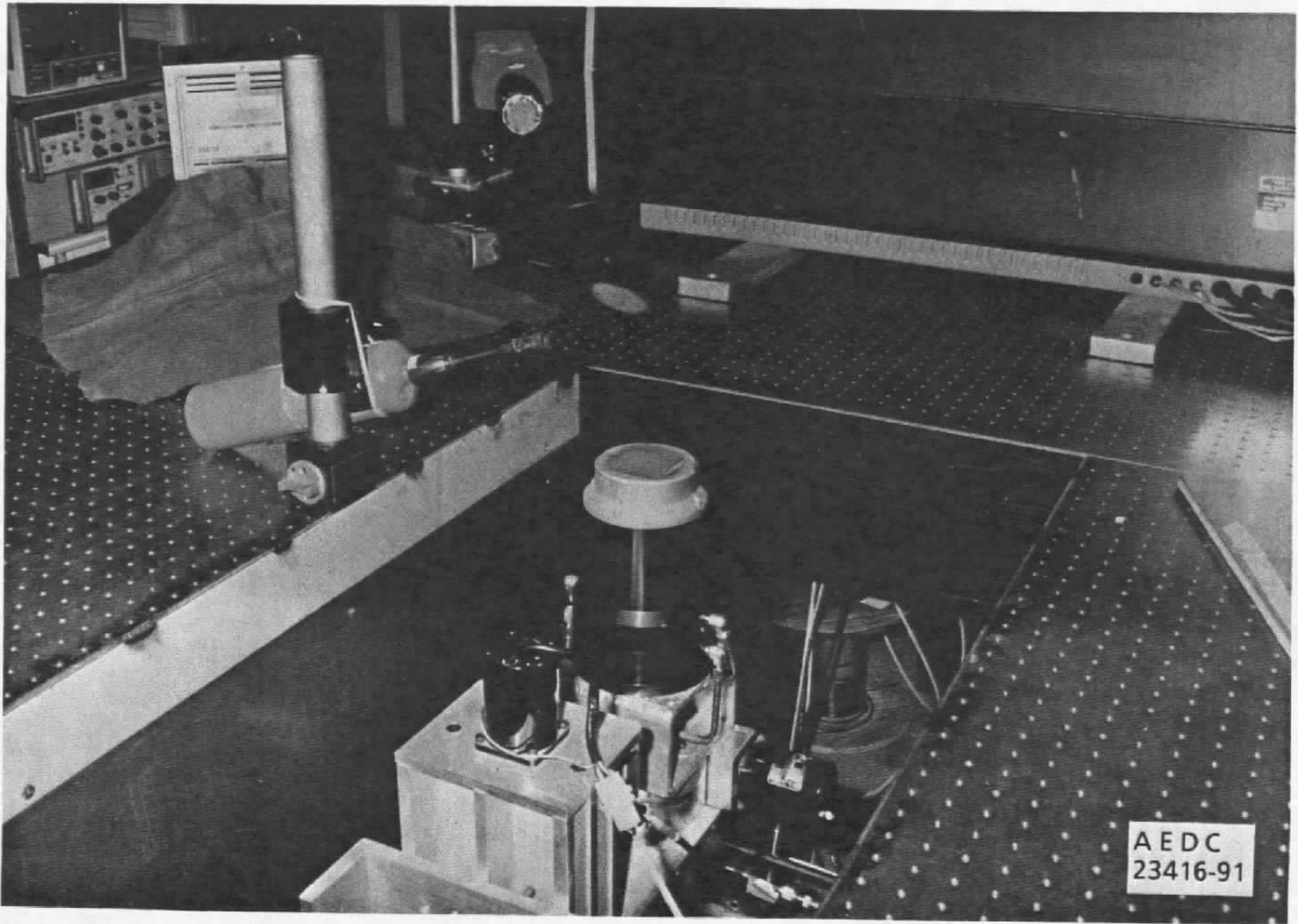
Figure 2. Photograph of flat flame burner and tomography experimental setup.
