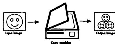
Figure 1. A copy machine that makes three reduced copies of the input image.
