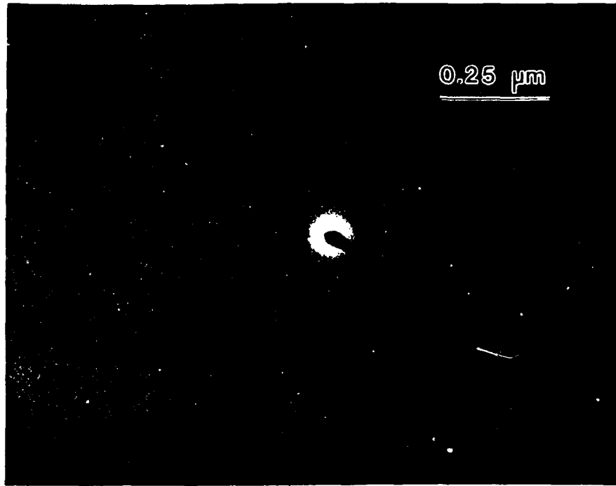
Figure 19. A TEM micrograph of a selected area diffraction pattern of the glassy phase in the \text{CaZrO}_3 grain boundary.
