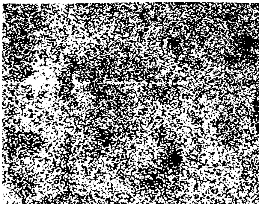
Figure 34b. Zirconium dot map of the outer surface of dry-pressed \text{CaZrO}_3 after vaporization at 1850^\circ\text{C} for 2 hours.
